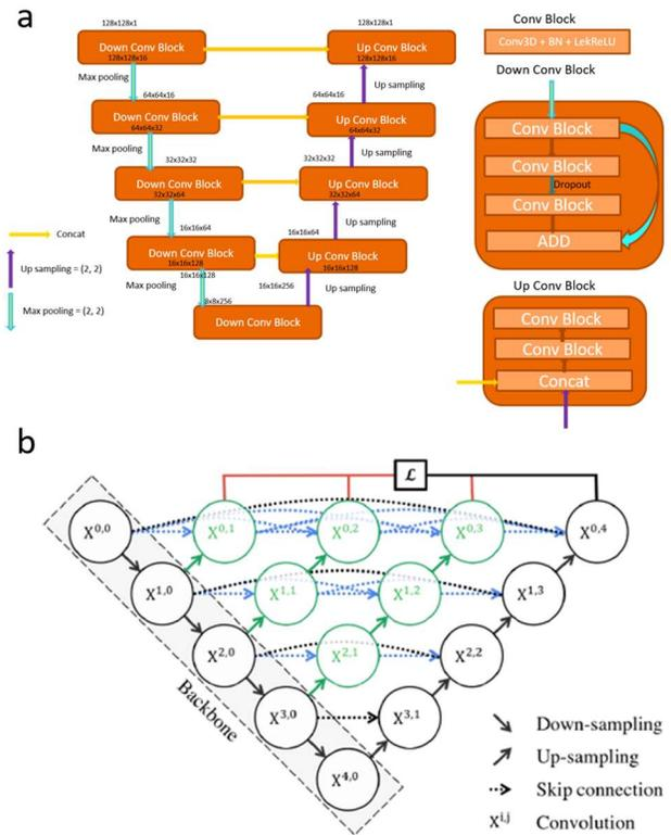
**Fig. 2. A)** U-Net used in first stage. **B)** UNet++ architecture with skip connection and deep supervision used in [15]
